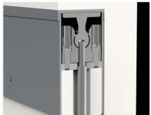
TRACK CUTAWAY
